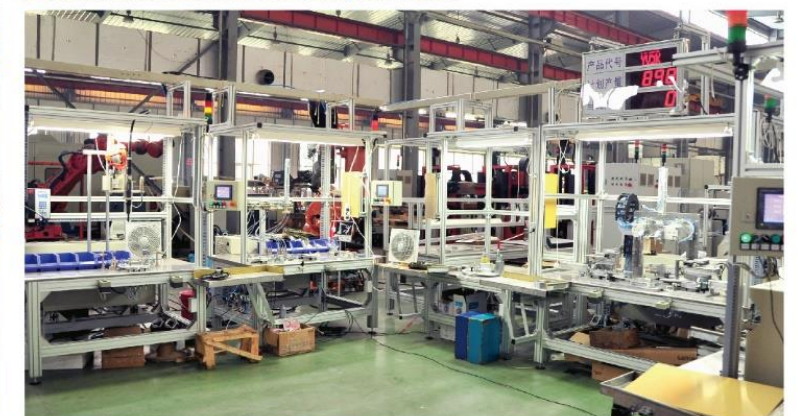
鼓式刹车自动装配检测生产线 Drum brake Automatic Assembly & test Line
